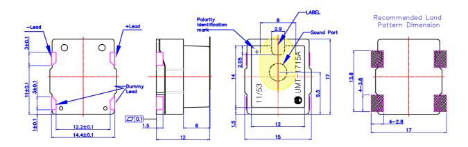
Tolerance: ±0.5mm Unit: mm
